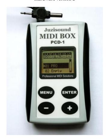
Juzisound PCD-1 breath controller is functional analog of Yamaha breath controller BC-3 + MidiSolutions box for analog to midi conversion – but this design is more modern and flexible!
